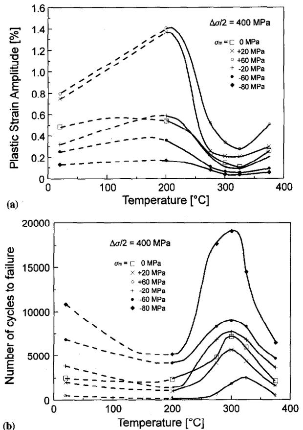
Fig. 1. Influence of temperature on the plastic strain amplitude (a) and on the number of cycles to failure (b) at six different values of mean stress.
