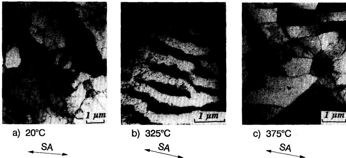
Fig. 3. TEM micrographs comparing the dislocation arrangements established in tests with zero mean stress at different temperatures. SA denotes the stress axis.
